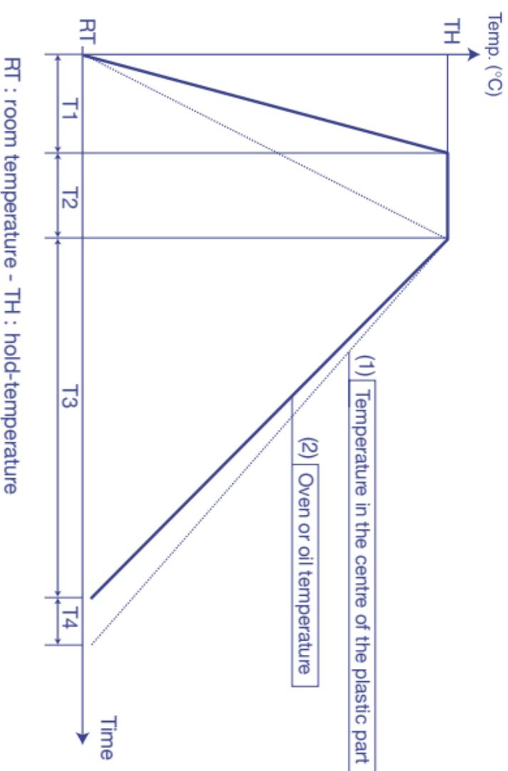
T1: heat-up time (heating rate: 10 – 20°C/hour)
